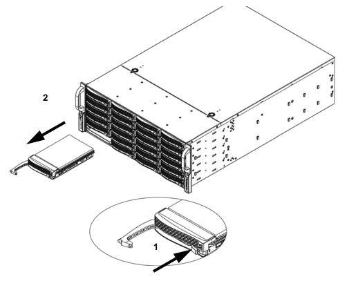
Figure 1: Removing the hard drive.
